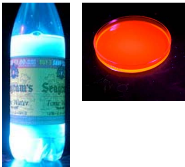
Figure 2. Left: Fluorescence of tonic water. Right: An acetone solution of chlorophyll under direct UV irradiation.
